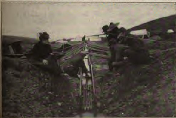
Placer mining in Alaska. The sand and gravel is washed down through a long trough which has slats across the bottom. The water carries the sand and gravel away, and the gold, being very heavy, is caught by the slats and picked out by hand.
